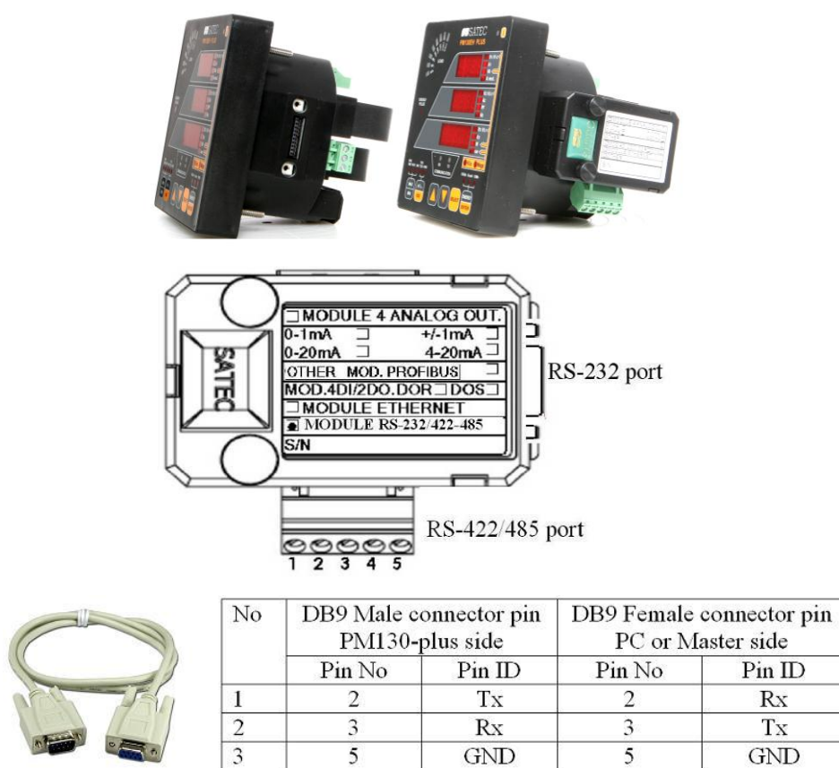
Figure 2-30: COM2 RS-232 connection
